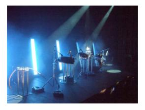
One of robots plays numerous pipes, and rapidly spins to create Flute-like sounds, which are generated while the air goes through them. These pipes are different lengths according to the pitches one desires. As it spins faster, the pitches become higher as following an overtone series.
