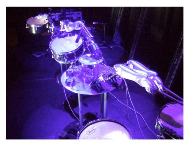
The robot has a special sort of springs to imitate a human muscle. Each holds a mallet at the end of his arm.
